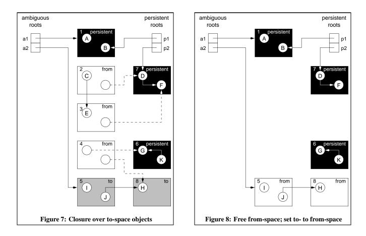
The mostly-copying *stabilize* procedure is sketched in Figure 2. We illustrate each phase of its operation with an example (Figures 3–8). Figure 3 shows the initial heap configuration for the example. As for mostly-copying garbage collection we begin by promoting from from-space to to-space all ambiguously-referenced pages (line 16). In the example, this results in the promotion of page 1 (referenced by ambiguous root a1) and page 5 (by a2), as depicted in Figure 4.
